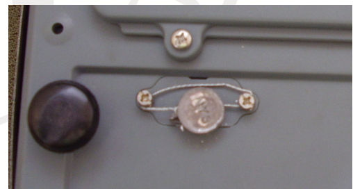
Calibration access via lead wire seal
